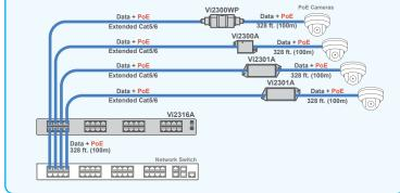
The Vi2316A and Vi230XXs can be used to connect multiple PoE cameras at extended distances
